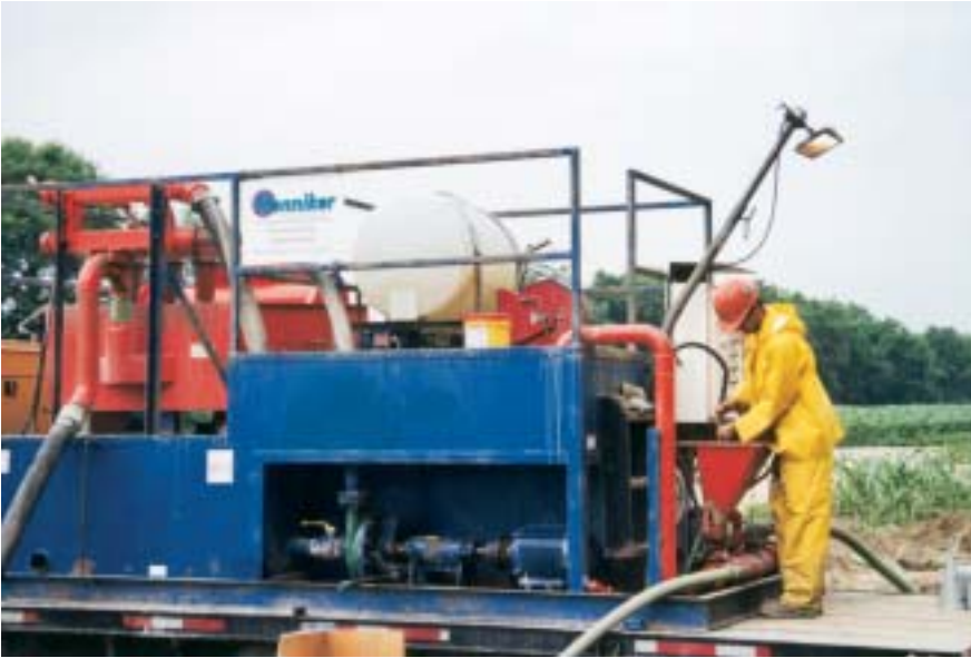
Above: HDD owner Jeff Martin mixes drillers' mud in American Augers recycler.
